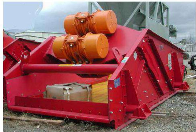
Figure 6 Vibrating dewatering screen
